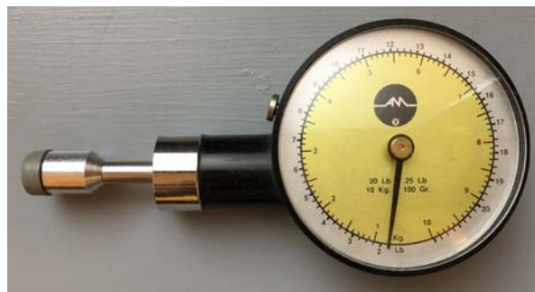
Figure 1.1. Algometer, used to measure pain thresholds of Tender and Trigger Points in test subjects with myofascial pain and fibromyalgia expressed in Kg/cm 2 . Equipped with a pressure distributing surface, it can be used to measure the amount of force performed by the test subject and is expressed in Kilograms. The arrow in the figures below indicate where and in which direction the device was placed to measure the resistance of the 1RM (resistance maximale) force exerted by the test subject. Note: Strength was measured through making use of a Wagner Pain Test™ Model FPK Algometer with a pressure pad.
